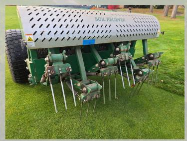
The soil reliever penetrates the greens 10 inches deep as you can see the irrigation flag (2 pictures below). Not only it penetrates, it fractures the clay bottoms. This will create a pathway for water from the surface into the drain tiles 12 inches deep. When we got 1 inch rain after we aerated the greens, the water came out of the drain tiles very rapidly. No puddling on the surface which means reduced the risk for ice damages.
